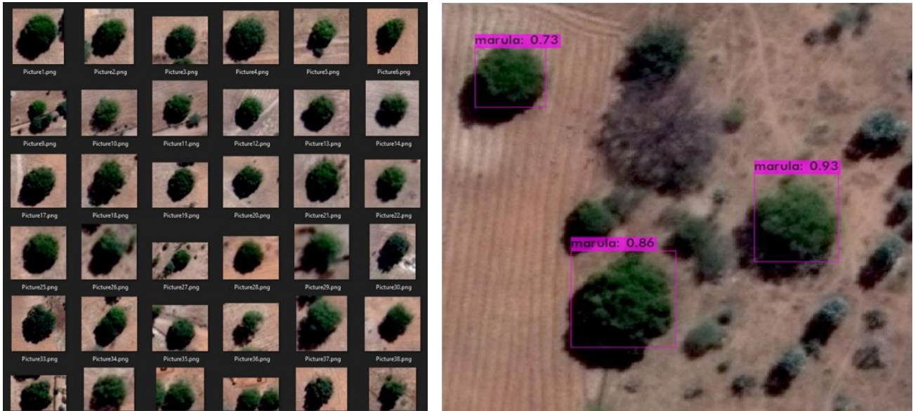
Figure 8: Examples of training set images (left) and the classifier in action (right) where it correctly identifies only marula trees in image.
