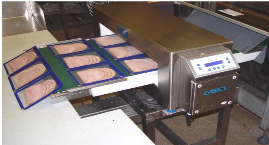
A typical metal detector, controlling metal hazards
