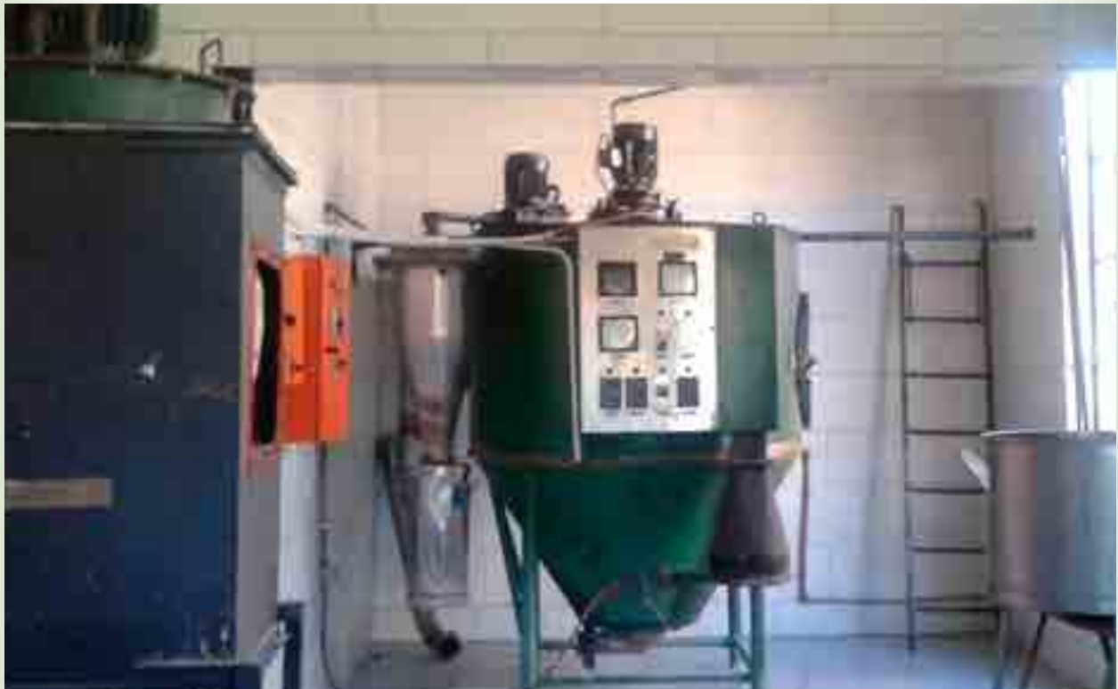
Spray dryer for spray drying aloe bitters
