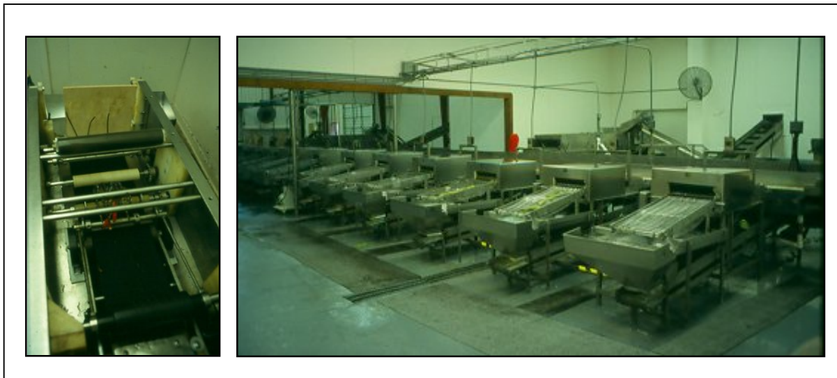
Figure 2.15: Mechanical filleting of Aloe vera leaves. On the left is a close-up photo showing the roller and conveyor belts. The photo on the right is of some of the filleting machines in the factory. (Photo from B-E. Van Wyk).
