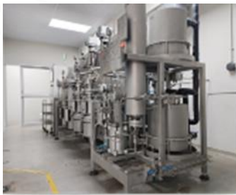
Supercritical CO 2 extraction equipment
