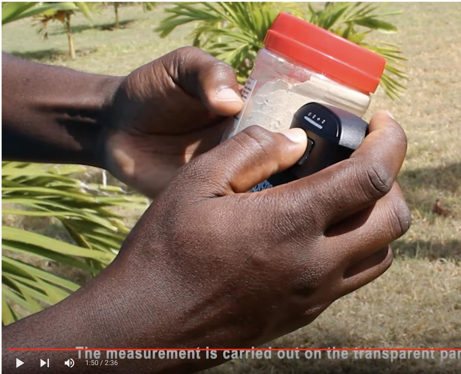
Baobab research: Using Near-infrared spectroscopy to determine baobab fruit powder quality
